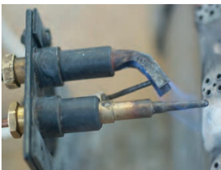
Pilot flame enveloping the tip of a thermocouple
